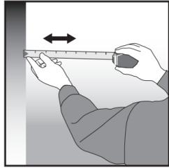
**1.** Measure the surface to be covered and calculate the number of panels needed.
