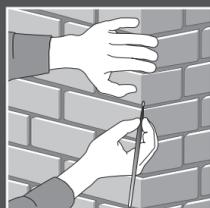
**F.** Once the filler paste is dry, paint the joint with Panespol special paint. Finish off by applying Panespol's ferrous oxide coating to give a perfect result.
