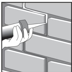
**5.** Once the whole wall has been covered with panels fill the joints and screw holes with glue-paste.
