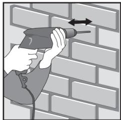
**3.** Fit the panel to the wall and drill through the panel directly into the wall using a 6mm drill bit. Put the screw into the wall-plug and introduce both into the hole in the panel. Push and screw them in until the panel is securely fixed (e.g. "Fisher" 6mm wall plugs and 4,5 x 40 screws are recommended). Use as many screws per panel as are needed.
