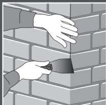
**E.** When the joint is filled, remove any irregularities in the paste with a fine brush.
