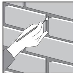
**6.** When filled, remove any irregularities in the paste with a fine brush. Once the paste is completely dry (approx. 24 hours), paint the joints and screw-holes with Panespol special paint, to give a perfect finish.
