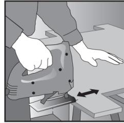
**2.** When starting the work, cut one side of the panel to get a completely straight edge.
