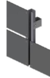
GENIETETES/ GESCHRAUBTES PLATTENSYSTEM AUF OMEGA-PROFIL
