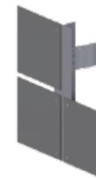
GENIETETES/ GESCHRAUBTES PLATTENSYSTEM AUF T-PROFIL
